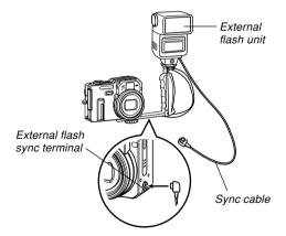
When attaching an external flash unit to the camera, you should also purchase and install a gripped bracket that can be secured to the camera's tripod hole.
